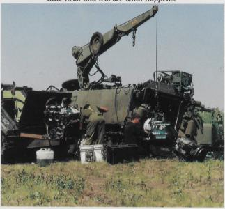
Exercise Rendezvous '89 — Maintenance Platoon personnel replace a power pack in an M-113. "The connecting rod connects to the piston ... or is it the valves?"
